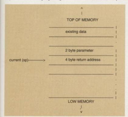
Figure 1: Position of the pushed stack parameter after the subroutine call message 'Please type your name.' It would, however, be useful to create a subroutine that could display any required text message.
